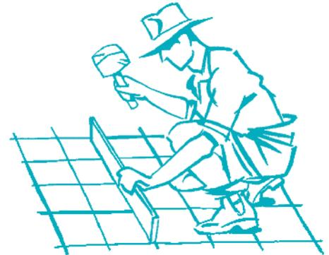
For driveways it is recommended that a minimum of 3 passes are carried out with a mechanical plate compactor. Bedding sand should generally compact approximately 10mm (1cm).
